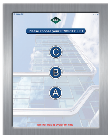
7 - Priority travel only with transponder card - lift freely selectable
